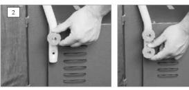
2. With the mill set on the hopper (as shown in letter a. above). Attach the legs via the threaded knobs (e).
